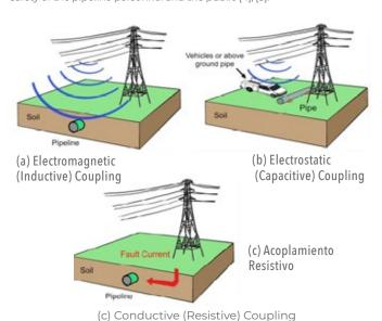
Figure 2: Types of AC Induced Interference on Pipelines
